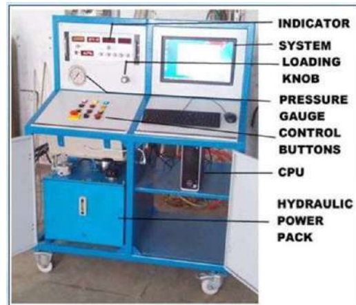
Frame control Panel
