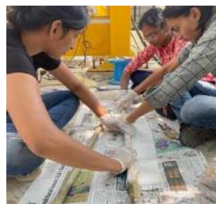
(a) Coating of epoxy resin
