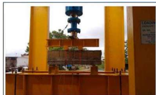
Testing of Beam
